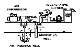
bisected by a railroad right-of-way, two separate remediation systems were specified. To the north, only air sparging was needed to address the dissolved phase plume. To the south, air sparging was augmented by soil vapor extraction to address contaminated soils above the water table. For this purpose, IES developed the system shown in Figure 1.
