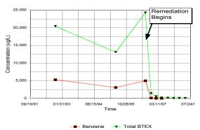
Approximately 1,600 pounds of gasoline were removed and groundwater BTEX concentrations were reduced by 91 to 100 % in each of the effected monitoring wells after 21 months of operation. Figure 2 illustrates the trend of groundwater concentration observed in one of the deep monitoring wells.
